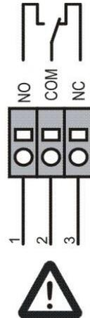
The fault relay is designed for a maximum voltage of 24V AC or 30V DC with a maximum current of 1A. Due to this fact (control voltage <50V), the all-pole mains isolating device according to EN 60204-1 for the connection cable of the fault relay can be dispensed with. The operator of the system must ensure that no control voltages >50V can be measured on the electronics after the system / fan has been disconnected from the mains.
